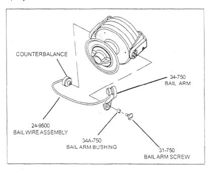
After unscrewing the counterbalance attached to the bail wire, attach the counterbalance included in the kit. Now attach the kit's manual pickup bail arm using the reel's bail arm screw and bushing. Be sure to insert the tag end of the bail spring into the hole of the bail arm. Also be sure the screw and bail arm bushing are in their proper places. If in doubt, consult your owner's manual.
