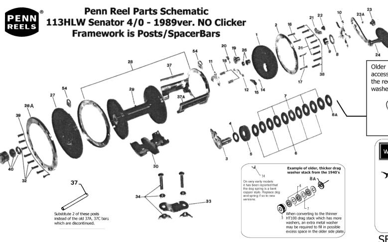
Older reels had drags accessible from outside the reel, using the 140 felt washer and the 136 collar/cap.
