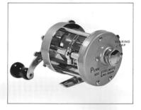
The left side spool bearing cap is located at the center of the left side plate. It is adjustable so that excessive end play of the spool can be taken up by turning the cap clockwise.
