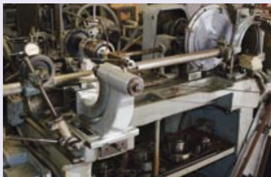
SCALING DOWN THE MOLD TO CUT THE DIE
